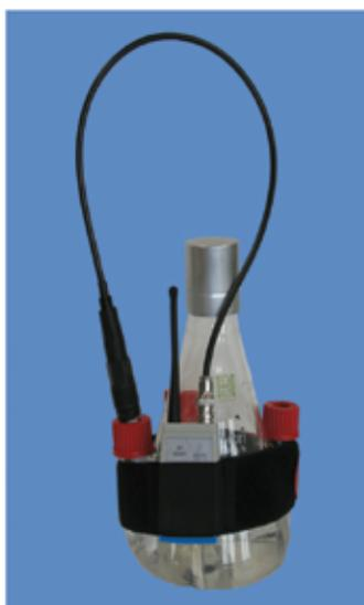
The best solution to measure physical data in closed systems (with contamination risk) or on moving platforms in laboratories or for outdoor measurements is the SENBIT® - radio system.
